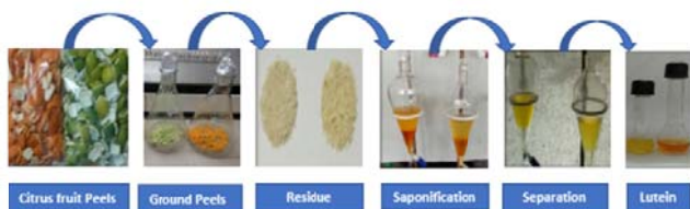
Figure 1 Extraction of Lutein from Citrus Peels by Maceration
